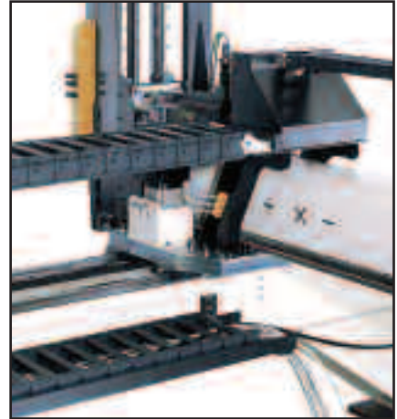
Rack and pinion gear on all 3 axes (models 1500 and higher)
