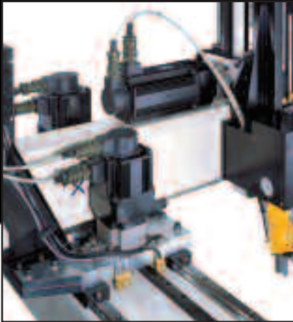
3-axis synchronized movement CNC servo motor drives
